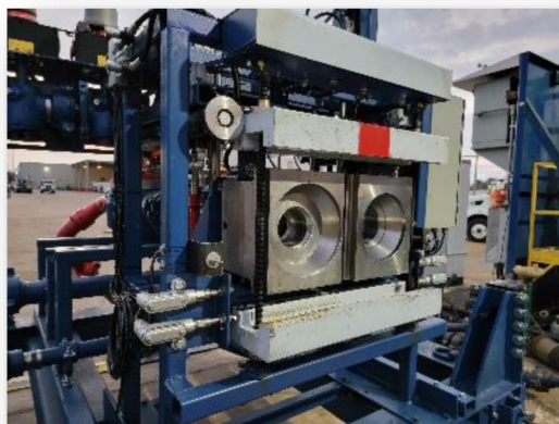
Figure 3—First Prototype of Automated Pump Swapping Skid
