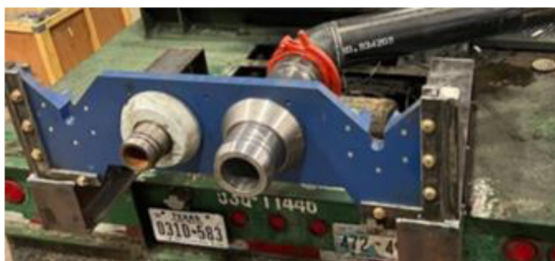
Figure 18—Modified frac truck showing the plate with two subs
